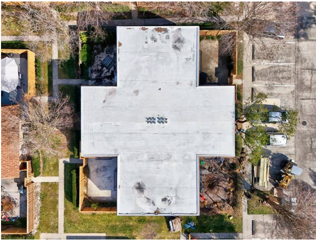
ROOF - CONCRETE WITH TPO COVERING
