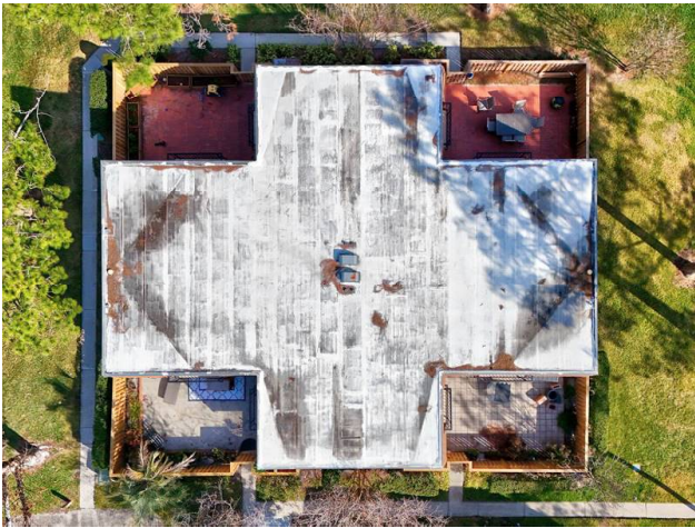
ROOF - CONCRETE WITH TPO COVERING
