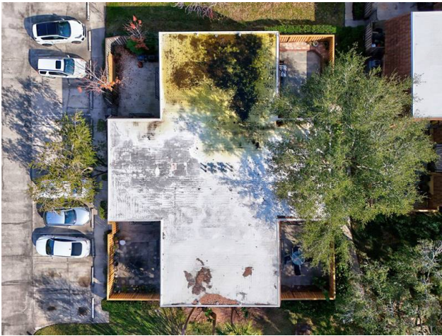
ROOF - CONCRETE WITH TPO COVERING
