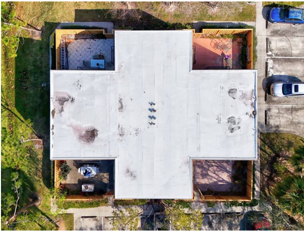
ROOF - CONCRETE WITH TPO COVERING
