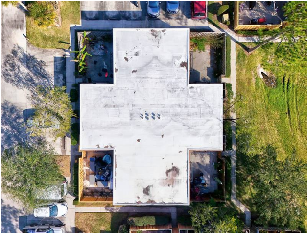
ROOF - CONCRETE WITH TPO COVERING
