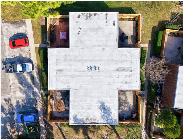
ROOF - CONCRETE WITH TPO COVERING
