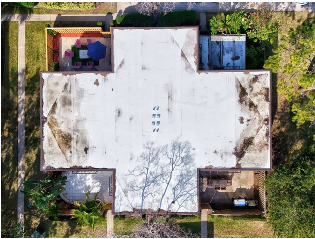
ROOF - CONCRETE WITH TPO COVERING
